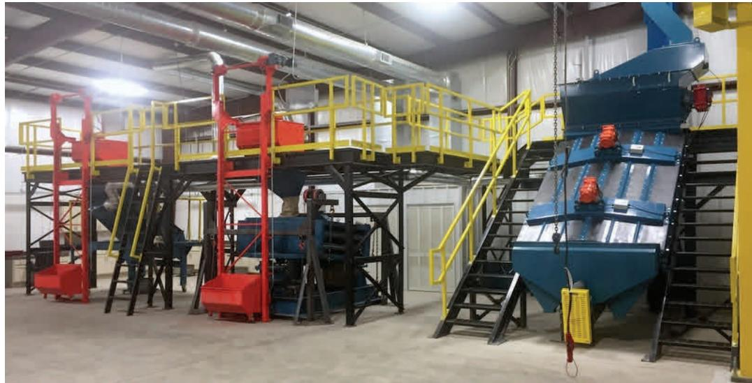
J&H will do the task of determining which wire cloth mesh for J&H Screen machines is most appropriate for your application. We have set up a research and test lab with two batch loaders and one continuous loop process screen for evaluating the performance and efficiency of any customer product.
