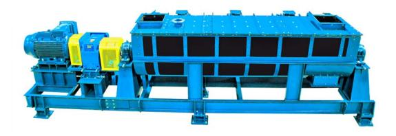
The Spinden Reactor is a paddle/pin mixer designed for continuous granulation of raw materials and recycle slurry to generate DCP and MCP as desired.
