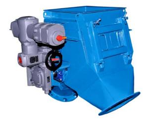
of material splitting or material distribution needs. Built with two or three discharges, our valves will handle from 50 to 800 tph and up of dry, loose material. Actuators position diverting blades or buckets in order to divide or divert the input stream of material as required for downstream demands. Actuator power feed can be electrical or pneumatic in both fixed position and in modulating versions.
