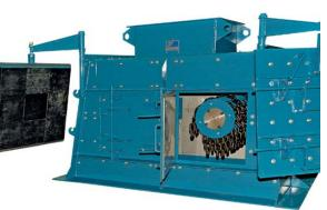
The J&H HD Chain Mill is driven by two electrical motors ranging in power from 25 to 100 hp each. Built in three different designs with widths ranging in six-inch increments from 24" to 36" according to the models, available in tonnages up to 100 tph.
