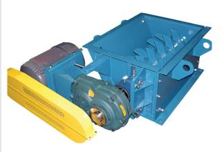
The J&H Lump Breaker is a compact machine designed with short, hardened tool steel teeth mounted on a rotating drum passing through an AR comb system. The rotor is driven by a shaft mount speed reducer in conjunction with Mill & Chem motors ranging in power from 10 to 50hp, depending on breaker capacity.
