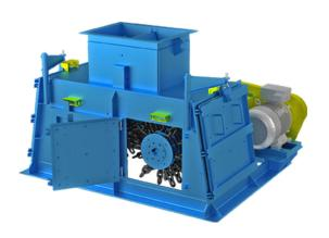
The J&H HD Chain Mill is driven by two electrical motors ranging in power from 25 to 100 hp each. Built in three different designs with widths ranging in six-inch increments from 24" to 36" according to the models, available in tonnages up to 100 tph.
