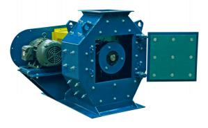
The J&H single rotor crushing machine is driven by one electrical motor ranging in power from 5 to 15 hp. There are two designs available each customizable to your specific needs.
