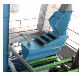
The J&H Velocity Breaker is designed to improve the operation of and extend the life of a J&H feeder/distributor by reducing the impact and speed of loose, dry product material into the inlet of the feeder.
