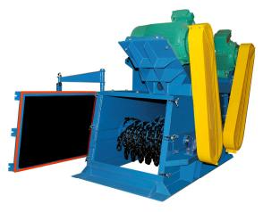
The J&H HDF Chain Mill is a dual rotor crushing machine driven by two electrical motors ranging in power from 25 to 125 hp each. Both rotors are equipped with a series of special hardened steel chain strands that are rotating in opposite directions, such apposing velocities generate a centergistic crushing zone.
