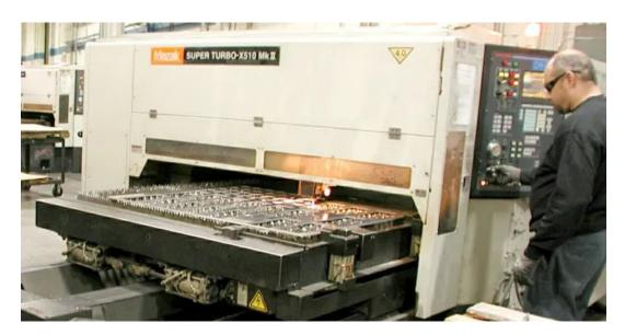
J&H Equipment uses some of the most advanced technologies for fabrication of our machines and parts. Items are cut using any one of five computer controlled laser cutters and automated loader which, as shown above, allows lasers to work through the night when scheduling demands it. Plate thickness from gauge to 1" can be cut into any shape required.
