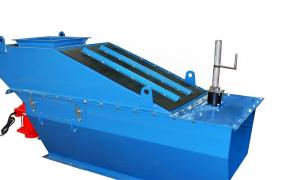
The J&H Feeder is a totally enclosed machine with a static housing and an internal stainless vibrating pan. The machine bolts directly to any J&H screen.
