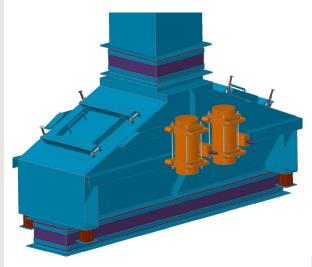
The J&H Vibrating Body Center Feeder is a totally enclosed machine in which the entire body and internal spreader pan vibrate as a unit. The machine bolts directly to and is supported by any J&H screen. It is mounted on four proprietary J&H vibration isolation buffers.
