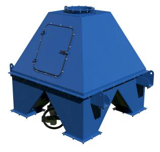
J&H Multiport Rotary valves are individually designed and engineered to accommodate customer requirements of plant layout, chute size and orientation, and type of product material. Built with a body of carbon steel, the valves are coated with a durable, industrial powder coat. Internal chutes are made of carbon or stainless steel. Feed and discharge port flanges designed to match customer chute work.
