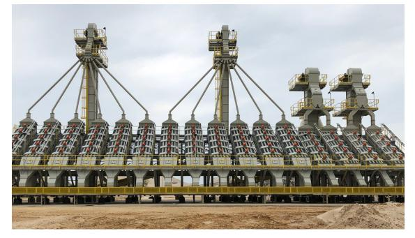
J&H offers a full range of screen support structures for all types of J&H Screens. The structure is designed to fully support the weight of the screen, hopper, and feeder while providing necessary access at all inspection and maintenance points.
