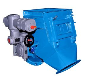
J&H Material Diverters accommodate all types of material splitting or material distribution needs. Built with two or three discharges, our valves will handle from 50 to 1000 tph and up of dry, loose material. Actuators position diverting blades or buckets in order to divide or divert the input stream of material as required for downstream demands. Actuator power feed can be electrical or pneumatic in both fixed position and in modulating versions.
